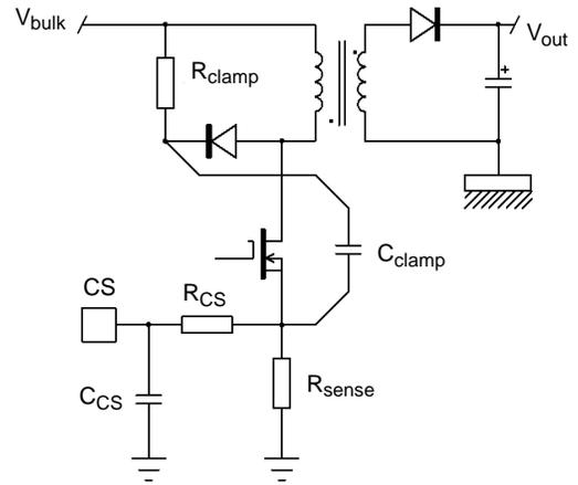
Figure 2. Fly-back Converter
