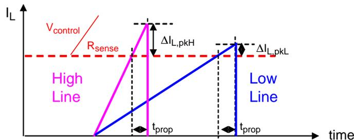
Figure 8. Propagation Delay Effect on Peak Current
